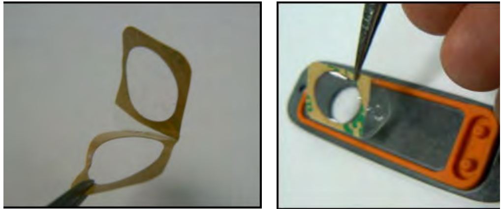
Figure 5. Removing the Backing from Prolene Window (Left) and Applying Window to Bracket (Right)
