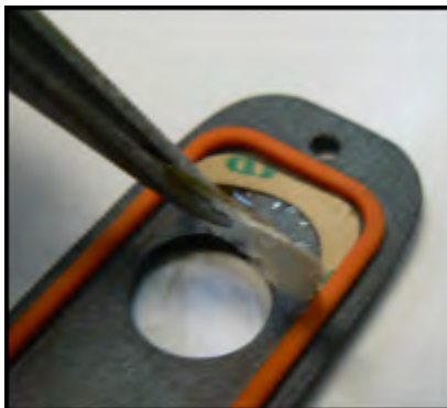
Figure 2. Removing the Old Window
