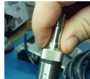
Properly completed—black ring uncompressed
