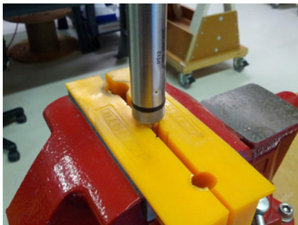
Cabled Sensor—gripping on swage
