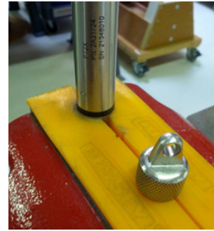
Cableless Sensor—gripping on knurled area
