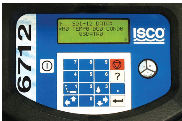
The 6712 Controller is also an SDI-12 data logger, and has many optional capabilities. Please contact your Teledyne ISCO distributor for more information.
